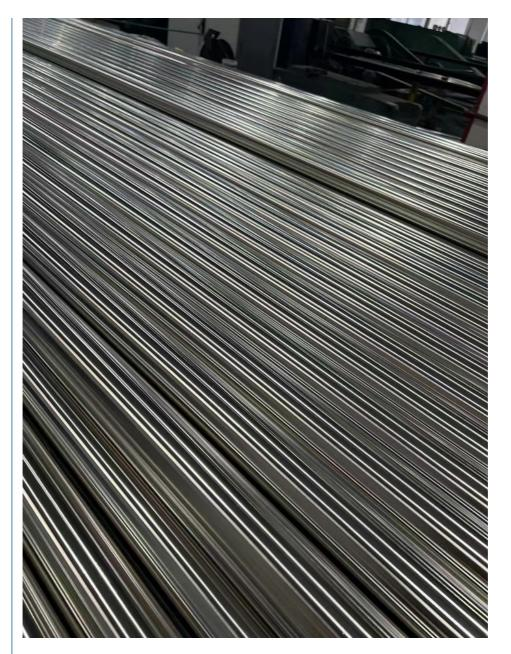
**Tensile Requirements – Stainless Steel 310S/310H:** Tensile Strength (KSI): 75 Yield Strength (KSI): 30
